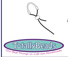
Step 3. Pull the tigertail tightly around the wire protector and push the crimp as close to the wire protector as possible. With your pliers, gently push the crimp flat to secure in place.
