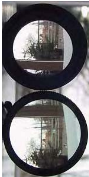
comparison of the exit pupil Baader Eudiascope and ADPS f = 25\text{mm}
