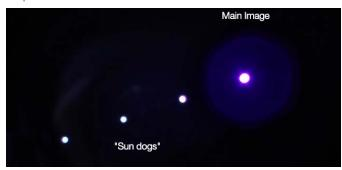
If you were to take a - very short - glance at the sun through the K-Line-filter in combination with Astro Solar Photo Film, you would see some asymmetrical, very dim "sun dogs" far away from the center of the image. They are caused by the tilt of the filters. With parallel filters, these reflections would all overlap and destroy the image quality. But since all reflections are directed to the side, you can image the centered UV-Sun through your telescope.
