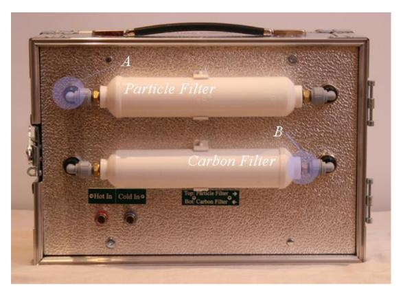
At point A you can feel with your fingers a small black ring. Press down on the ring and carefully release the grey elbow. Repeat at all four points.
