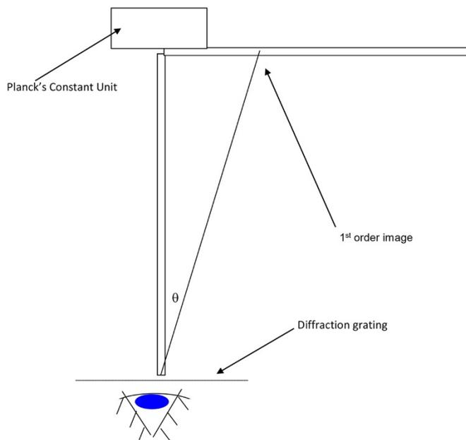
Using the formula  $n\lambda = d\sin\theta$ , the wavelength of the red light may be calculated.  $d$  is the diffraction grating spacing =  $\frac{1}{500,000} = 2 \times 10^{-6} \text{m}$
