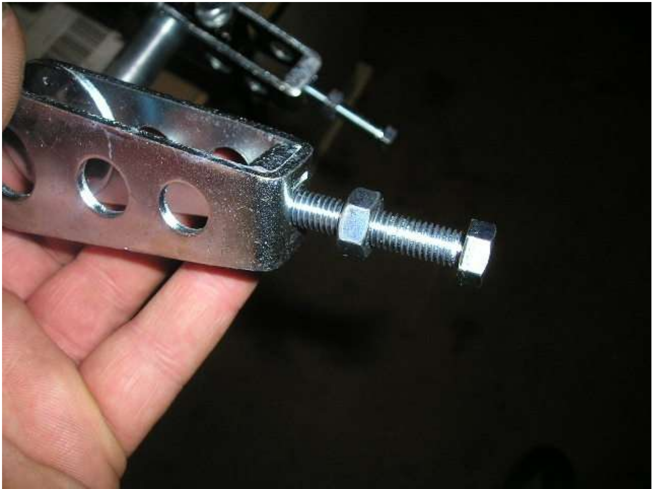
The rear brake rod is a genuine one, very rare these days. Then i fitted the new rear footrest.
