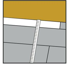
**10.** Final row. Measure the width of the final row of boards The final row of boards must have a minimum width of 50mm and a minimum 15mm expansion gap must again be left at the edge.
