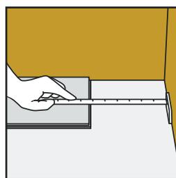
**4.** At the end of the first row, place a 15mm expansion gap spacer against the right hand wall or skirting board, and measure the length of the last board to fit.
