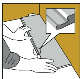
**1.** First board, first row. Place 15mm expansion gap spacers against the walls or skirting boards at the left hand end, and back long edge, of the first board and position the board end against the wall. The tongue on the back edge of the board should be against the spacers on the facing wall.
