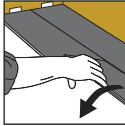
**8.** Place the board tight to the short end of the previous board and fold down in a single action movement, continue in this manner for the following boards and rows.
