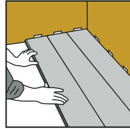
**9.** After 2-3 rows. Adjust, if needs be the distance between the front wall or skirting and the flooring edge and ensure adequate numbers of 15mm spacers are in place to keep the flooring edge a minimum 15mm away from the wall or skirting at all points along this edge.
