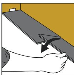
**3.** Fold the board down with a single action movement to locate the header joint. Continue with the next boards in the same manner.
