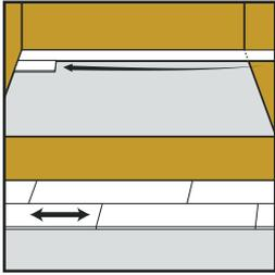
**6.** Second row. First board, min length 500mm. Use the off cut from the final first row board, (if it is 500mm or longer) to start the second row of boards, Again leave an expansion gap of 15mm against the left hand wall or skirting board. Ensure a minimum 150mm distance between the short end joints of the boards laid in the previous row and the new row being laid. No adhesive is required on the joints of this row of boards.
