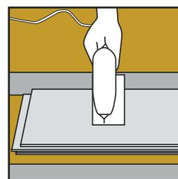
**5.** Cut the last board to length – hardwood face turned down if using a jig saw or hardwood face upwards if using a hand saw.
