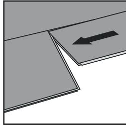
**7.** Second board second row. Locate the long edge tongue of the board into the long edge groove of the previously laid row. Do not glue these boards simply lay them dry using their drop loc edges.
