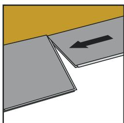
**2.** Second board, first row. **Place a bead of PVA adhesive along the short header joints only of this first row** of boards and locate the board end into the short end of the first one
