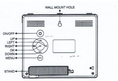
Press Menu button to enter screen menu. Use UP and DOWN button to highlight the line to apply changes. Use LEFT and RIGHT button to underline the text for adjustment. When underlined, use UP and DOWN button to make changes. Press MENU button to close changing mode.
