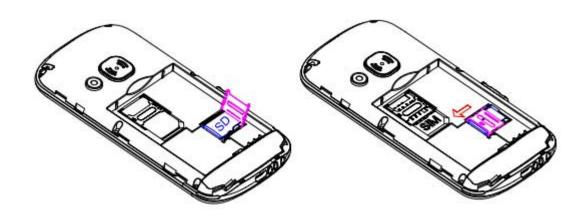
3.Insert the SIM card by carefully sliding into the holder. Make sure the SIM card's contacts are facing inwards.
