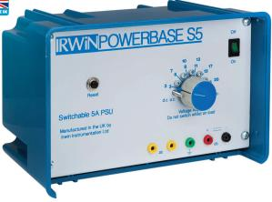
The Powerbase S5 is a heavy-duty power supply offering 0-12V ac and dc outputs. Both outputs are selected by a rotary switch and may be used simultaneously up to a combined output current of 5A.
