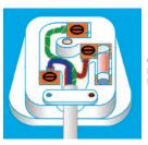
Green/Yellow wire to the terminal marked: Blue wire to terminal marked: Brown wire to terminal marked: E (Earth) coloured Green/Yellow N (Neutral) or coloured Blue L (Live) or coloured Brown
