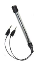
The IRWIN search coil is designed to detect and measure a.c. magnetic fields. It is composed of a 3,200 turn coil on a 20mm former. The coil is mounted on a Perspex tube handle and the connections are terminated with 4mm plugs. The axis of the coil is parallel to the handle. The coil should be orientated so that the direction of the field to be measured passes through the coil i.e. up through the handle
