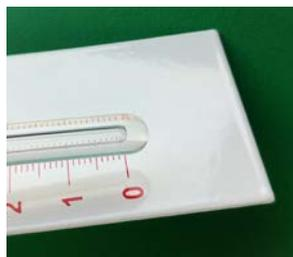
**N.B.** Before carrying out the experiment ensure that the base of the capillary tube is aligned with the zero mark on the base plate.
