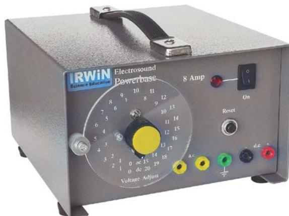
The Powerbase is a heavy-duty power supply offering 0-15V ac and 0-20V dc smoothed outputs. Both outputs are continuously variable and may be used simultaneously up to a combined output current of 8A.
