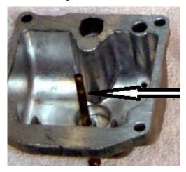
Our "Carburettor" trouble shooting guides covers how to check the float heights. Kawasaki state that the float height for the Z1 Z1a Z1b should be 24mm. For the later A4 and Z1000 models a range of 24 to 26mm is specified. People on the forums have even set the height as high as 28mm to get the fuel height right. We start by aiming at 25mm, but achieving that can be a challenge.
