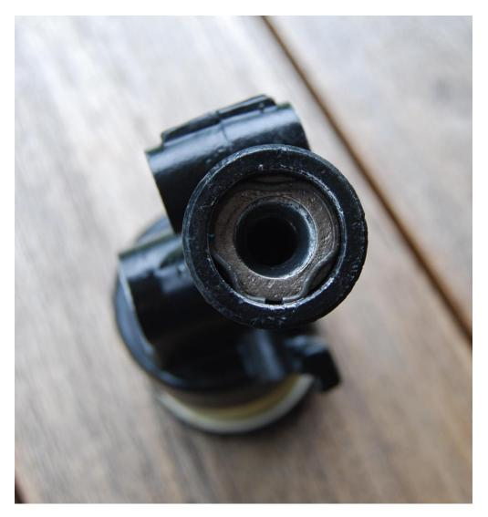
The clip and the washer are easy enough to remove, but the piston can be very stubborn. We have found that an M8 tap will fit in it very nicely. Having tapped it out, you can screw in an M8 bolt, put an impact wrench (if you have one) on the end of the bolt and give it a wiz. If you pull a bit at the same time the piston should come out. A little bit of heat may help but too much and you will certainly need a new seal.
