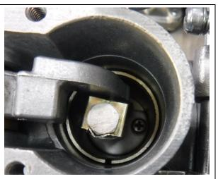
There are 2 screws that secure the slide to the bottom of the lifter; remove them and the slide will come out of the tops. The needle is then just tipped out.
