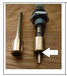
The effect that high ethanol levels in modern fuels have on the rubber components in carburettors is well documented. If the rubber in the end of the choke plunger (arrow on the right) goes hard and fails to seal the choke, allowing air to bleed past, then it is effectively running with choke on all of the time.
