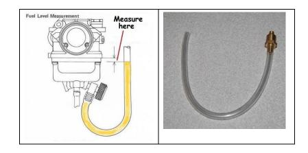
In theory the float height should be set using a manometer, or "float height adjustment tool". Carbs wear, patent float valves are a little different. There are lots of variables and this is the only way to be sure (eg, if you are still having over flow problems after setting the float height)
