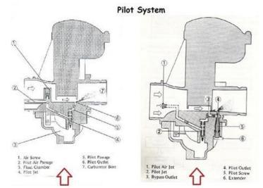
The average base line for the air screws is between 1 -1/4 to 1-3/4 turns out from lightly seated but given their age and possible wear they may be happier well above or below that. The usual procedure is to start with them midway at 1-1/2 turns out and go from there.
