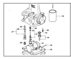
It has also been suggested that Erratic idle can be caused by one or more missing "O" rig that sits on the fuel screw shown as 32 in this diagram
