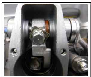
Remove the bolt that holds the slide lifter to the arm (this is a Z1 carb – 7mm bolt)
