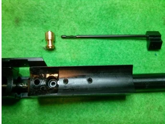
Once the magazine latch rod has been removed you can remove the brass transfer port. *There should be a rubber O ring either end of the transfer port, one may still be inside the air cylinder/hammer tube assembly (leave it there).*
