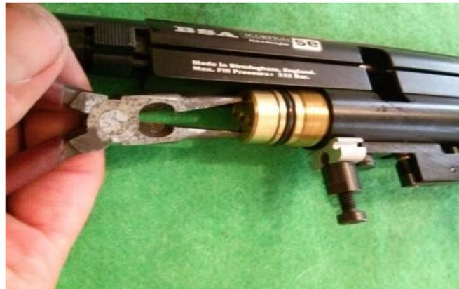
Once the lid/cover has been removed then pull out the internals and put the brass knockoff restrictor (16-6623) to one side, it is not fitted when a regulator is used. Refit the firing valve (16-6057) (*aka knock-off valve*) and the pre-load spring (16-6092) and cover/lid (16-6622). Now fit the new HuMa regulator onto the brass firing valve, it only needs to be hand tight.
