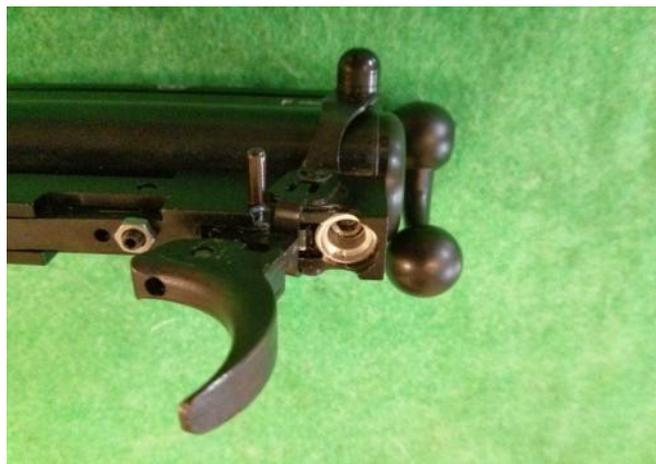
Now use a 3mm Allen/hex key to remove the front bolt from the trigger mechanism, *Some tactical models may have a little black plastic plug in the screw, you will need to pop it out to gain access to the bolt.*
