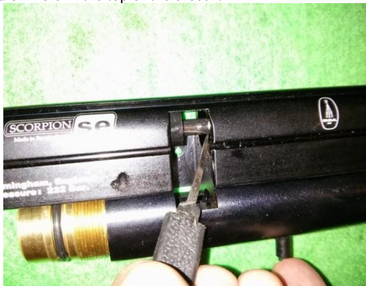
Use a 3mm Allen/hex key to remove (anti-clockwise) the cap head bolt that is now visible through the hole in the top of the breech, that was blanked off before carrying out the previous step.
