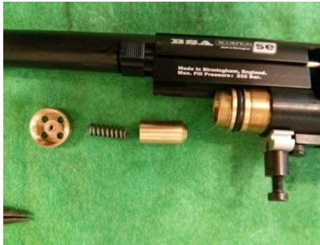
Fit the pressure gauge banjo (16-7690) onto the regulator being sure not to damage the O rings.
