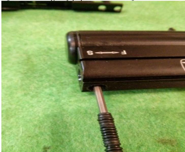
Use a small screwdriver/pokey device to push the little silver looking part that you can see inside the hole in the left hand side of the breech, next to the magazine slot. Pushing this will unlatch/unlock the pellet probe.
