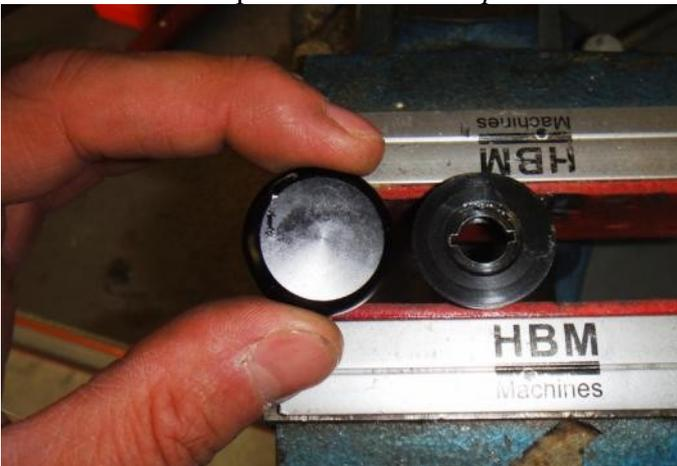
**Optional:** Remove the steel hammer spring guide (*top hat*) (16-6523) from the hammer tube and replace it with a plastic spring guide (available from the eShop). *Some rifles don't have spring guides fitted at all, don't worry about this, fit the plastic spring guide if you have one.*
