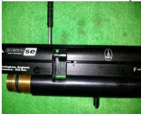
Turn the complete action over, while holding it together (*remember you have just removed the 2 bolts that hold that air cylinder/hammer assembly and breech block/barrel together!*).
