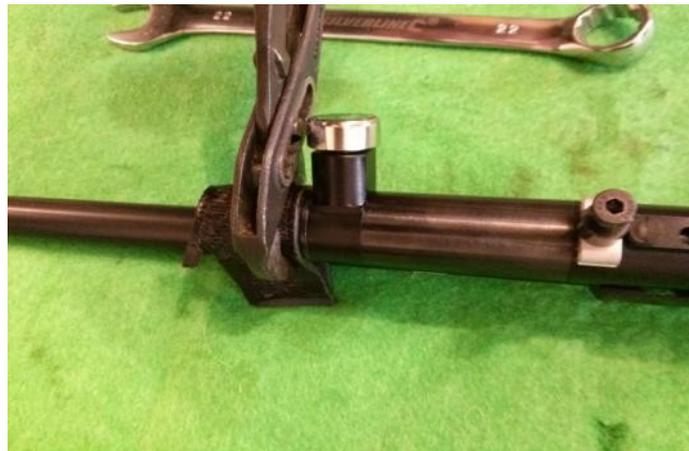
Once the air cylinder and the various adaptors etc have been removed you should have the brass firing valve body (16-7450) on show, remove the brass firing valve cover/lid (16-6622) (*looks like a pepper pot lid*).
