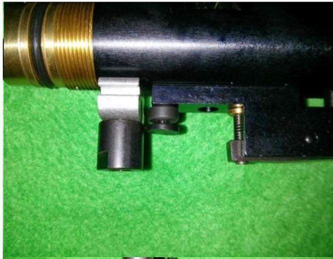
Use the same 3mm hex key to remove the bolt from the back of the trigger mechanism (through the blanking plug you have just drilled).
