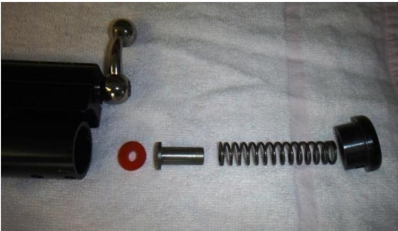
There is a black cap (16-6530) fitted to the power adjuster which needs to be removed to gain access to the power adjuster. There are a few ways of doing this:
