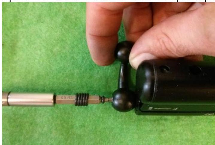
Use a flat screw driver to remove (anti-clockwise) the blanking plug (16-6728) on the top of the breech/scope rail. *They are normally fitted with Loctite, so can be stiff, a screwdriver that fits the slot well will be able to remove it nicely, a poor fitting screwdriver may cause a bit of damage to the plug.*
