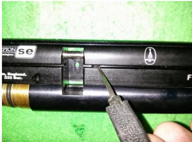
Use a screwdriver to push the probe and black plastic probe guide (magazine bridging guide) (via the magazine slot) backwards until you can see the bolt head of the forward breech fixing bolt, via the previously blanked off hole in the top of the breech.
