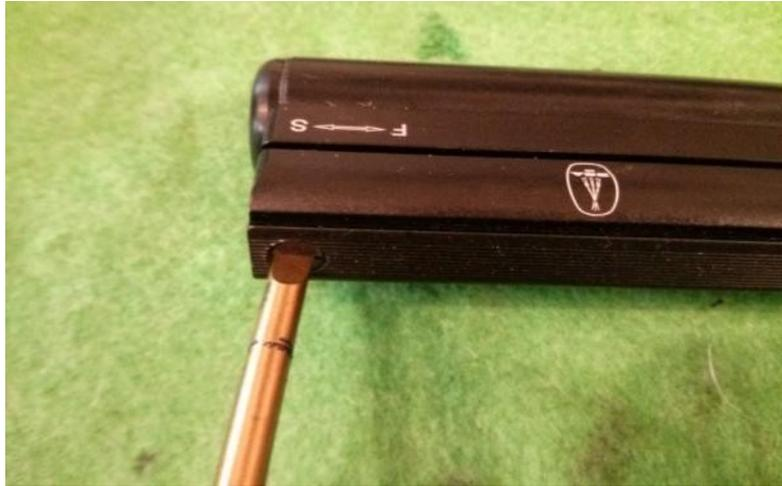
Use a 3mm Allen/hex key to remove (anti-clockwise) the cap head bolt that is now visible through the hole in the top of the breech, where you removed the blanking screw in the previous step. *Be sure to remove it completely or else the next step will be impossible. When this bolt is removed the black cap and power adjuster housing may pop out the back of the action.*
