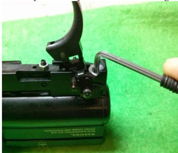
Remove the cocking bolt/handle using a 3mm Allen/hex key, be sure to support the head/ball of the bolt to avoid putting strain on the probe. The little bolt/probe extension should come off with the bolt handle, if not use a piece of leather around the extension and a pair of pliers to wiggle it loose.
