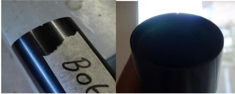
Following your mark on the valve body, file a small groove in the longitudinal direction of the screw-thread of the valve body.
