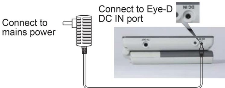
To charge the Eye-D, insert one end of the power supply into the charging port (labelled DC IN) on the top edge of the unit on the far-right hand side (when the screen is facing away from you). Then plug the other end into a mains socket and turn it on.
