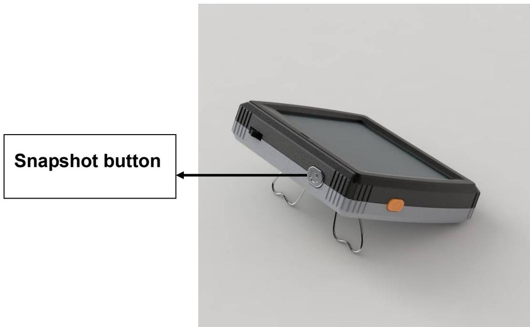
**Snapshot button:** The snapshot button allows you to take a temporary picture of a distant text or image, enabling you to bring the image closer to your eyes for easier reading.
