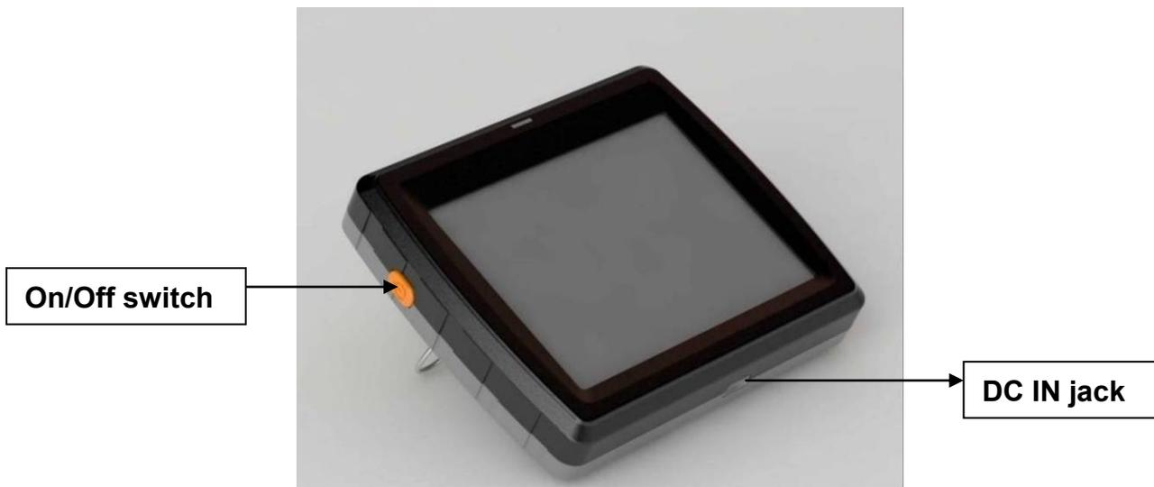
**On / Off switch:** Press the small round orange button for two seconds to switch the unit on / off
