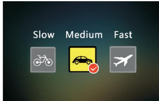
2. Press “+” button or “-” button to select the speed you prefer, and press Mode button to confirm. It will automatically exit to the setting menu (the first class). Short press the Freeze button to exit setting menu.
