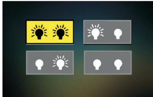
2. Press “+” button or “-” button to choose LED light status. By default, the LED lights are ON in near-view and OFF in distance-view mode.
