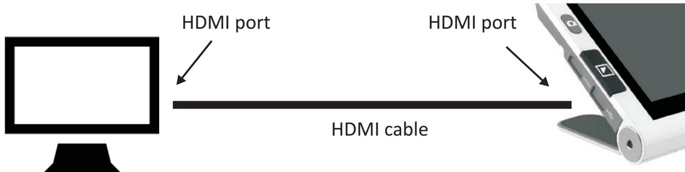
Once connected, the Snow 7 HD Plus screen will turn off automatically and enter HDMI output mode. And the contents of material will display on the monitor or TV.
