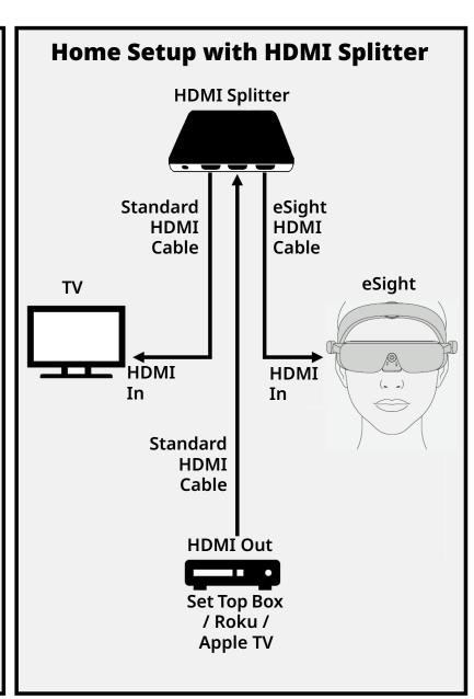
The eSight-approved splitter is an optional accessory that allows you to connect an HDMI video source to the TV and eSight 4.
