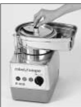
Next fit the appropriate slicing disc and screw the slicer on the motor shaft with the butterfly nut.
