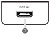
**DIAMI OUT:** Connect to your HDMI transmitter box or display to overcome the shortage of the power from the source.
