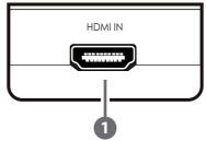
**PARTY IN:** Connect to the HDMI source equipment such as a Blu-ray player or an HDMI switcher/HDMI Splitter/HDMI Matrix.
