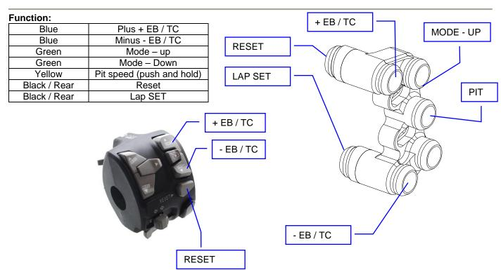
NOTE: Throttle twist grip must be OPEN for the +/- EB/TC functions to work
