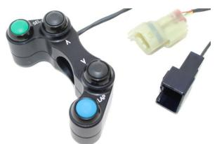
This 4 way left switch can be used with the standard right side switch or these matching right side switches
