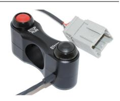
This switch includes the wires for the brake light switch, simply plug them into the 2 remaining pin locations of the 6 way connector block and lock in place with the connector latch. For bikes that do not need the brake light switch simply leave them off and close the connector latch.
