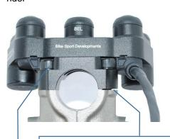
**0.5mm of gap** – Used for tightening the clamp. 21.5 > 22.2mm dia bar
