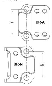
Standard 32mm spaced brake clamp
