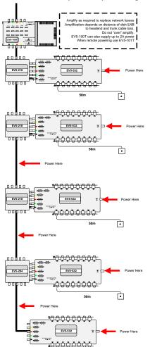
Where a "star" network is required the multiswitches can be connected to a splitter/splitters to form an equi-distant cable network. Each multiswitch will be provided with the same signal levels for equal performance. Calculation of the cable attenuation based on the cable lengths can determine the correct amount of amplification.
