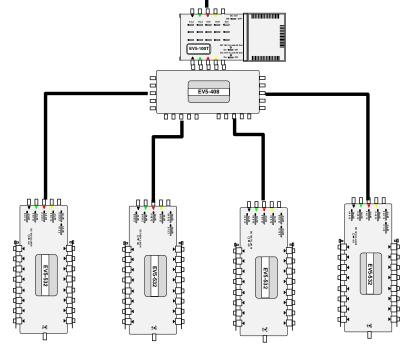
V5-EVO multiswitches have "stepped" gain outputs (shown in data above) to accommodate short and long subscriber lines with a 2dB step in each group of four (or eight on EV5-524 and 532) outputs. Gain is pre-emphasised to high frequencies to counteract the effects of cable slope attenuation.
