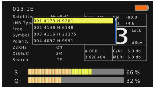
When a signal lock is reached, the buzzer will sound with fastest repetition. The signal quality bar is displayed on the LCD and the LOCK LED will light. Press [OK] on the search option to scan for channels on the selected TP. It will switch to the Program Page after the search is complete.
