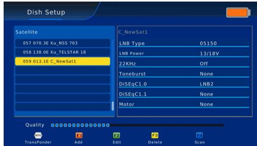
In the satellite list page, press [▲/▼] to select the required satellite channel plan. Press [F1] to add a new satellite with satellite name, longitude direction, longitude angle or band.
