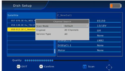
Press [GOTO] to access the TP list. [F1], [F2], [F3] & [F4] can be used to add, edit, delete or begin the scan of the selected TP. Press [GOTO] to return to the satellite list.
