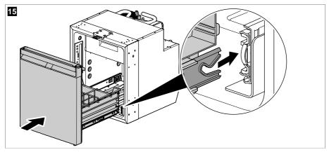
4. Slide the drawer open and closed several times to ensure that it slides easily.
