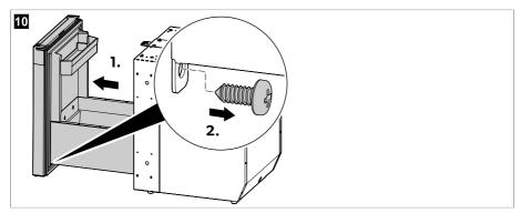
2. Remove the side panels. To do this, push the first side panel towards the cabinet to release it from the catch hooks (1.). Repeat the process on the other side with the second side panel.
