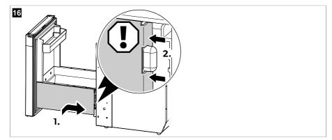
6. Fasten the screws behind the door on the side panel on both sides.
