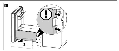
3. Push the lever on one side upwards and at the same time push the lever on the other side downwards and carefully pull out the drawer.
