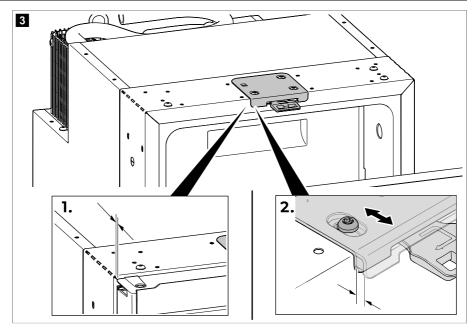
3. If the drawer opens or the opening gap is greater than 5 mm , adjust the door latch position until the opening gap is in the range 2 ... 5 mm ( Fig. 3 on page 12, 2.).
