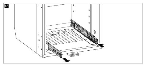
2. Align the groove of the extended cabinet rail with the guide of the corresponding drawer rail. Press the drawer rail onto the cabinet rail until the rails are connected and slide easily.
