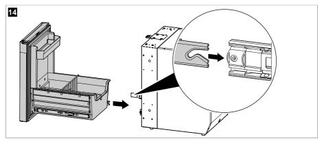
3. Carefully slide the drawer inwards on the connected rails and align the groove of the retracted cabinet rail with the guide of the corresponding drawer rail. Press the drawer rail onto the cabinet rail until the rails are connected and slide easily.
