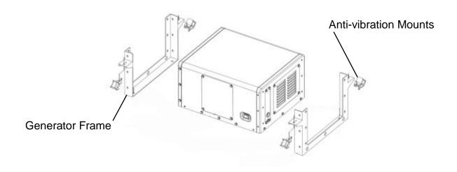
2.7 If using the slide out frame option, fix the anti-vibration mounting direct to the base of the generator then fix to the slide out frame.
