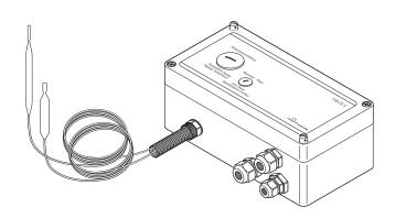
A surface sensing thermostat providing temperature control and temperature limiter in safe areas. The high limit cut-out prevents the heating system exceeding a preset maximum temperature should the control function fail to operate or an unsafe process temperature occur.
