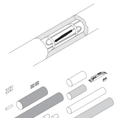
These splice kits are designed for the in-line joining of nVent RAYCHEM BTV, QTVR, XTV, KTV, HTV and VPL self-regulating heating cables.
