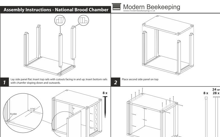
Nail side panels to end boards using 16 x 50mm round head wire nails,
