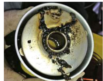
A filter clogged up with diesel sludge
