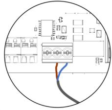
If the eSense signal is provided by using an external voltage this must be connected to the two right hand terminals marked "24-230V AC/DC in"
