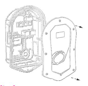
Step 3: Remove all 8 screws from the enclosure and carefully lift away.
