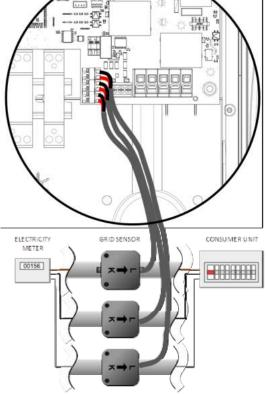
**SINGLE PHASE**: A CT clamp must be placed around the live meter tail as shown above with the arrow pointing towards the consumer unit.
