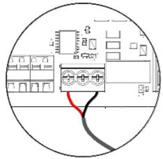
If the eSense input is provided using an external volt-free contact then this must be connected to the outer terminals marked "24V out" and "in"
