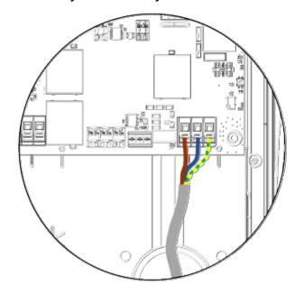
For single-phase installations, without the need for hardwiring an external CT, please follow the above diagram
