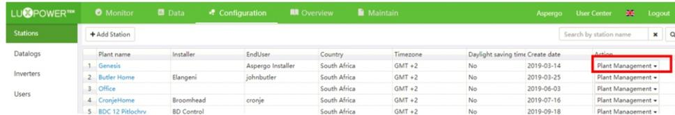
Step3. Setup Master and Slave for Parallel system. There should be only one master in the system. Set one inverter as master and the others as slave
