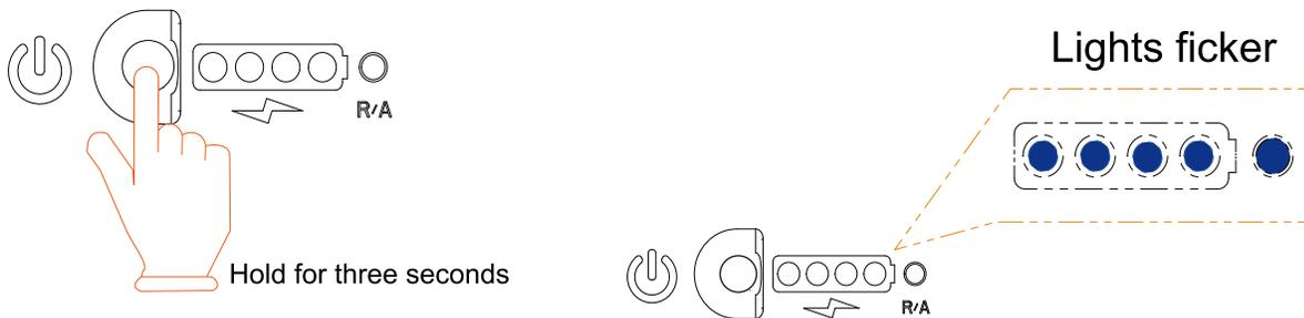
If the SOC indicators turn on and the RUN indicator flickers for five times, the batteries are powered on successfully and the communication between batteries works.
