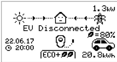
The EV is not connected to zappi.
