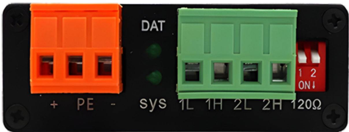
Figure 2.2 Location of power interface and CAN-bus interface
