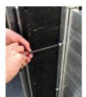
Now, using the T-Bar tool supplied, apply two full turns to the vertical compression screws.
