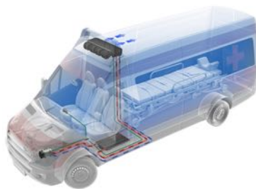
Integrated air-conditioning system
