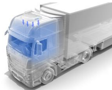
Parking air-conditioning system
