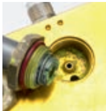
Sealant contamination in the A/C service unit without the use of the Recycle Guard
